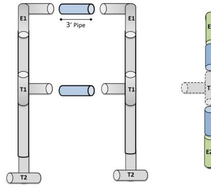
Gray: 2 elbows, 4 tees, 4 pipes (cemented) Blue: 2 pipes (not cemented)
